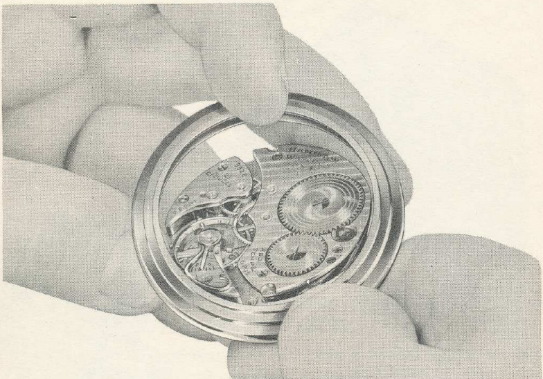
Figure 53 — Hamilton Pocket Watch — Case Screws Removed
